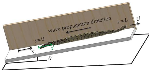
**Figure 2.** Schematic of the apparatus used to study rectilinear locomotion. Here,  $\theta$  is the inclination angle with respect to the horizontal. The front wall (not shown) is composed of Plexiglas. The ground coordinate frame ( $x$ ) and moving coordinate frame ( $x'$ ) are indicated by the arrows. The direction of wave propagation in rectilinear locomotion is opposite to the direction of motion. (Online version in colour.)
